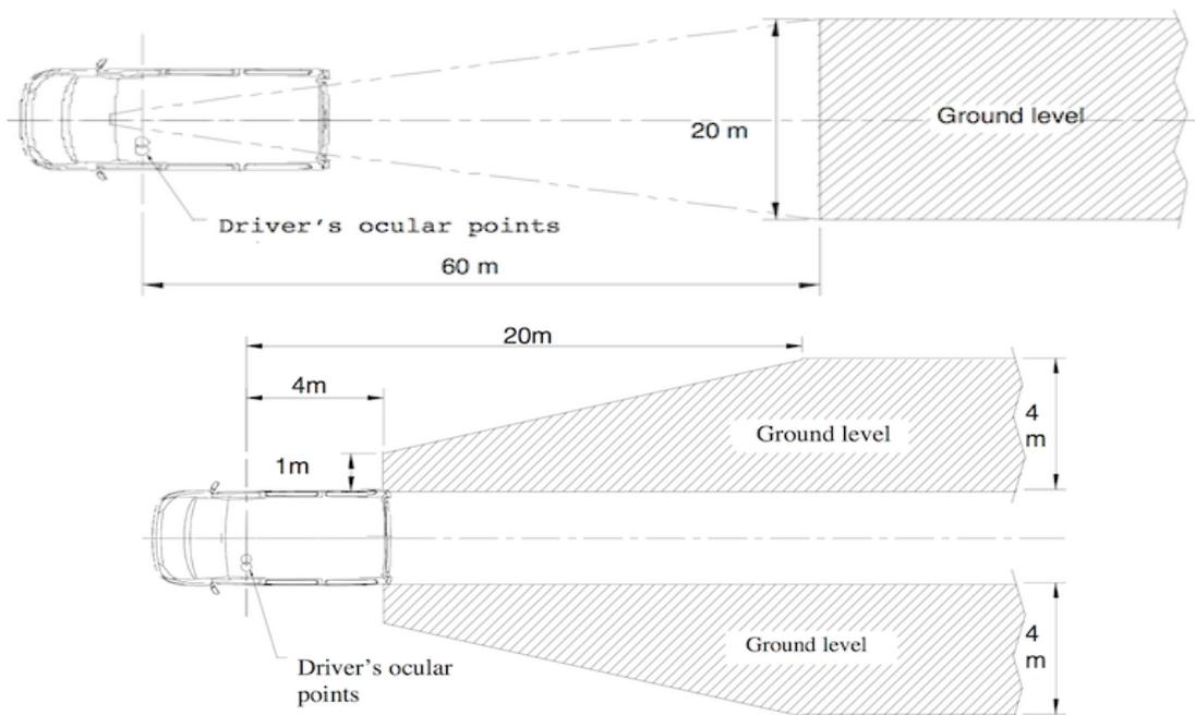
1.18.2 Rear vision systems may be electronic, mirrors, or both. Rear vision systems must operate whenever the solar car is in motion under its own power or about to be driven. Rear vision
